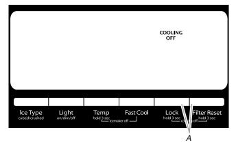
A. Press LOCK and FILTER RESET at the same time.
