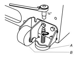
A. Leveling screw B. Front roller
